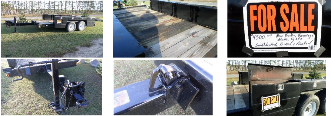
Tandem Axle trailer with pintle hitch, tilt, and tool boxes
